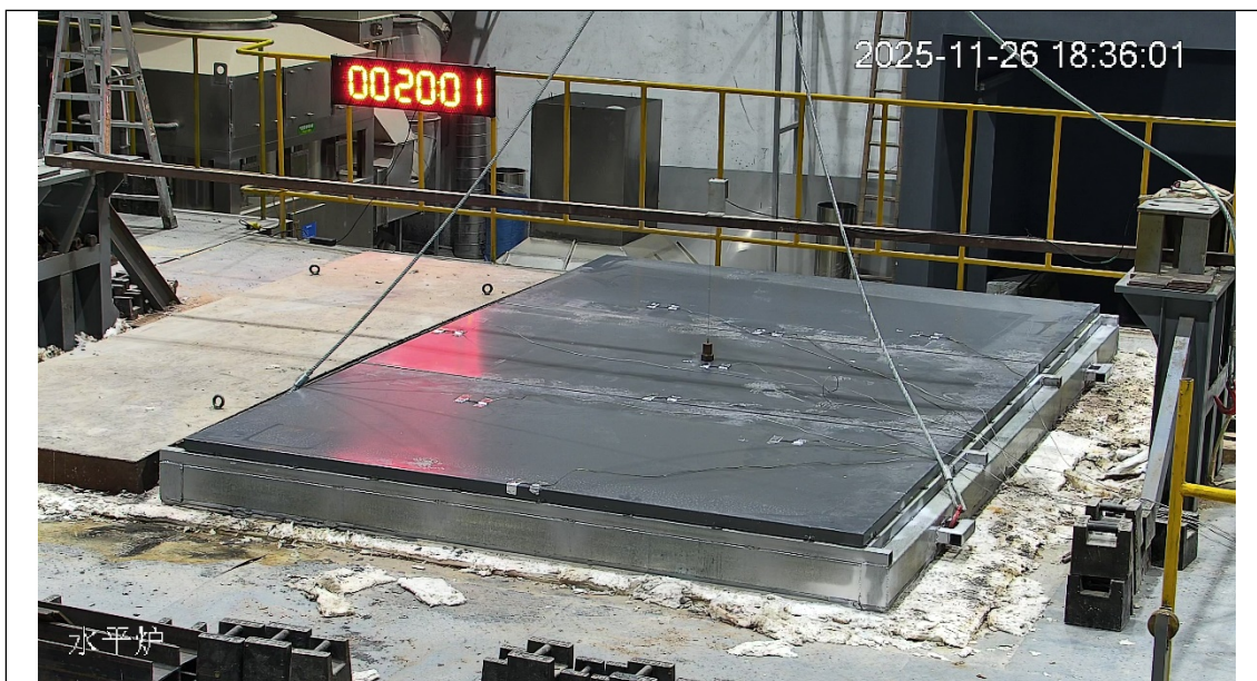
The unexposed side after 20 minutes of testing
