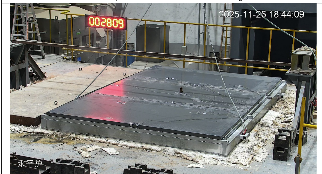
The unexposed side after 29 minutes of testing
