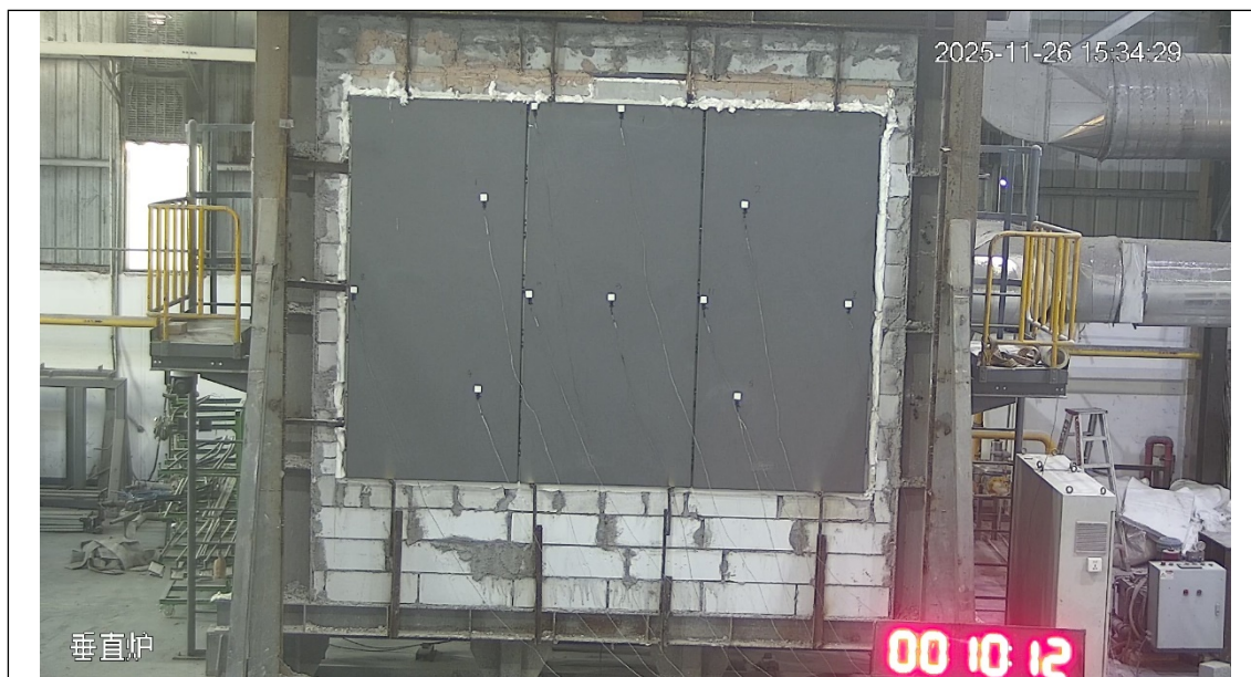
The unexposed side after 10 minutes of testing
