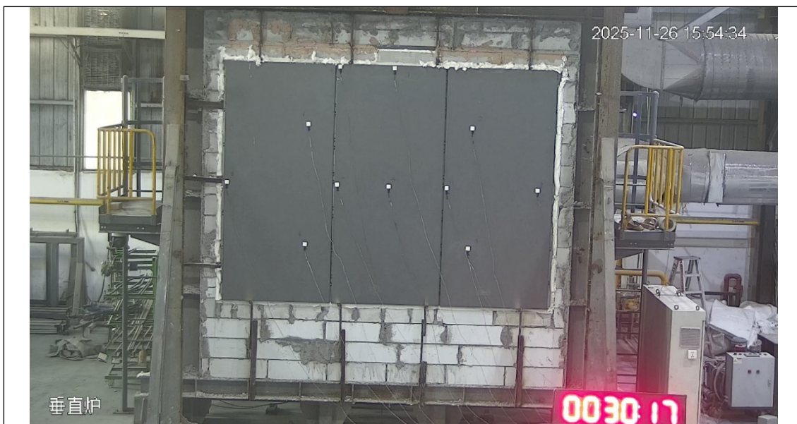
The unexposed side after 30 minutes of testing
