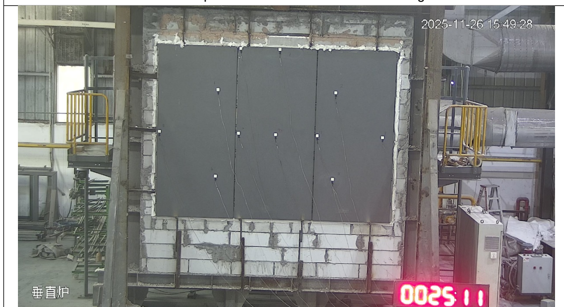
The unexposed side after 25 minutes of testing
